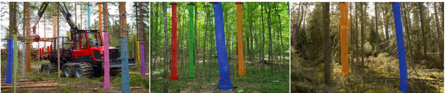
Fig. 4: Predictions on real images from ResNeXt-101 trained only on synthetic images. We observe that even with the reality gap, the model can still detect trees with high precision, but suffers from low recall rates.
