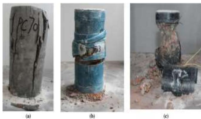
Figure 5 Failed specimens under compressive load (a) Plain (b) GFRP confined concrete (c) CFRP confined concrete [45]
