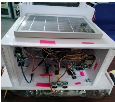
Fig -6: Integrated with Ultrasonic Sensor
