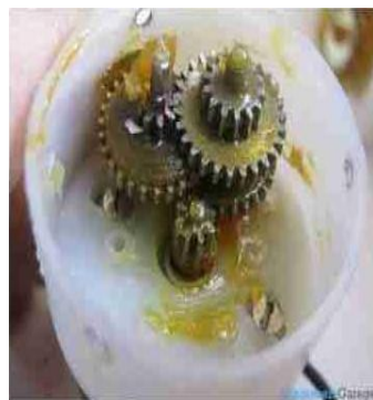
Figure7: Internal gearing of 12 v dc motor
