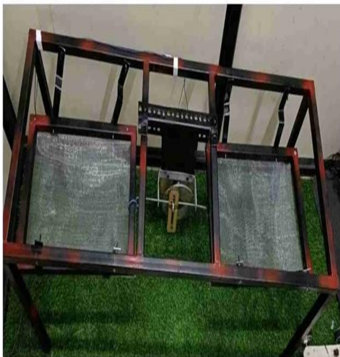
Figure 2: Two Way Sand Filter
