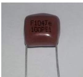
Fig 8. Bye pass Capacitor
