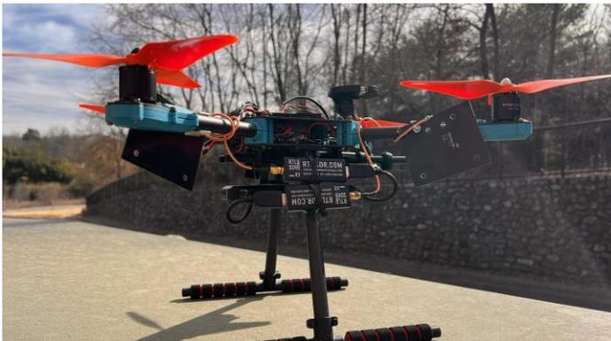
**Fig-9.** Configured drone with SDRs and associated components.
