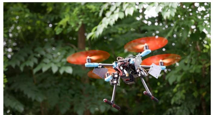
**Fig-11.** The AIMS SDR RF measurement and visualization system, drone mounted.
