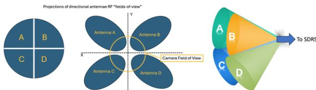
Fig-3. Directional antennae and companion visible camera fields of view.
