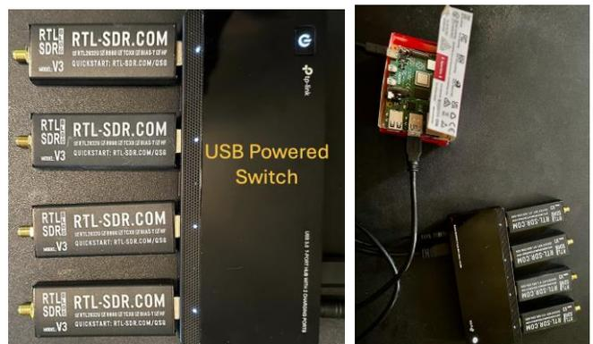
Fig-5. Optimized hardware configuration: RTL-SDR into powered USB Switch into Raspberry Pi3.
