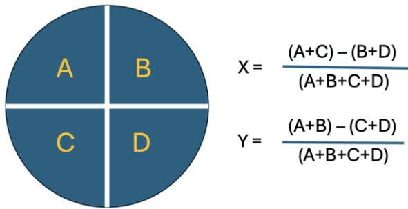
Fig-2. Optical quadrant detection centroid determination.
