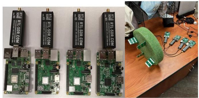
Fig-4. (a) Initial hardware configuration. (b) Directional antennas mounted in a Styrofoam disc.
