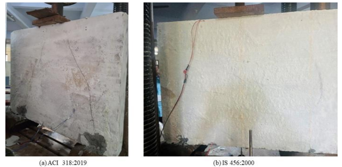
Fig-6: Diagonal Splitting Failure in The Beam
