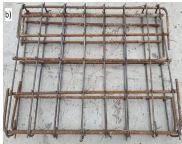
Fig-3: Reinforcement detailing of specimens a) ACI b) IS
