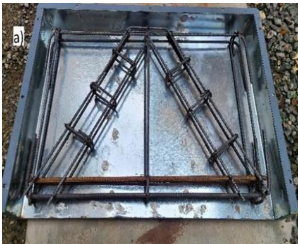
Fig-3: Reinforcement detailing of specimens a) ACI b) IS
