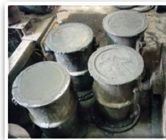
Fig-2: Casting of Cylinder
