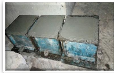
Fig-1: Casting of Cube
