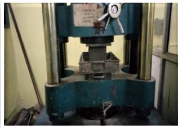
Fig-3 Compressive strength test in UTM
