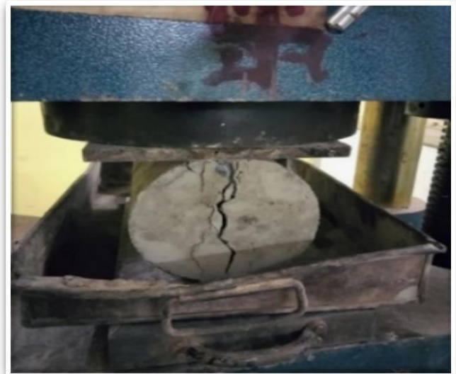
Fig- 4: Split tensile strength test in UTM
