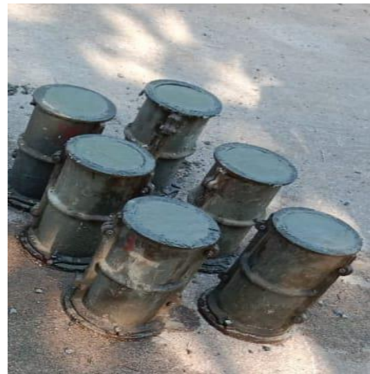
Fig-2: Casting of Cylinder
