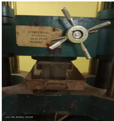
Fig-4: Compressive strength test in UTM
