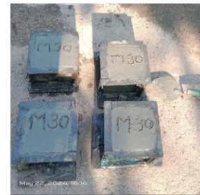
Fig-1: Casting of Cube.
