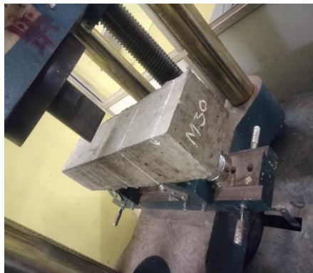
Fig-6: flexural strength test of concrete in UTM
