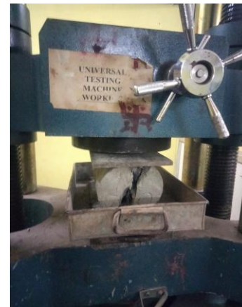
Fig- 5: Split tensile strength test in UTM
