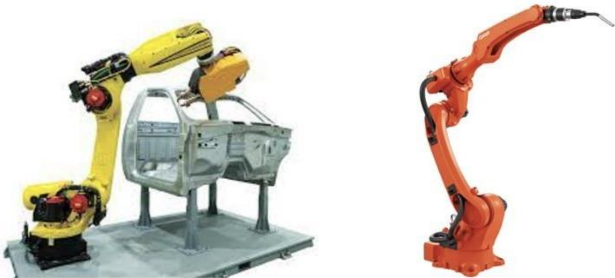
Fig -6: spot welding robot on the left [35] and arc welding robot on the right [36]
