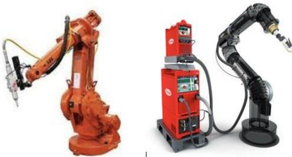
Fig -7: laser welding robot on the left [37] and plasma welding robot on the right [38].
