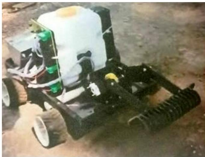
**Fig -5:** Prototype of Agriculture System
