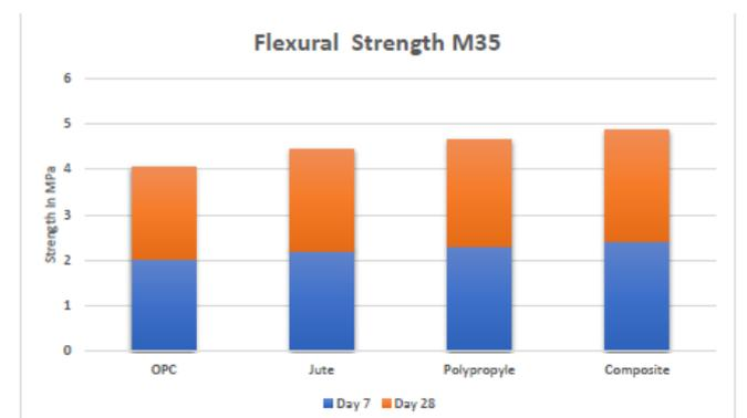
Fig -3.2 Value of Flexural Strength M35
