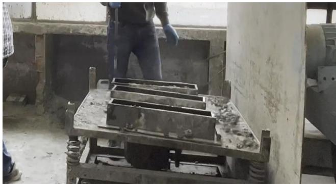
Fig -2.5 vibrating table
