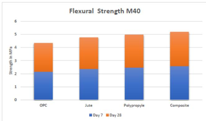
Fig -3.3 Value of Flexural Strength M40
