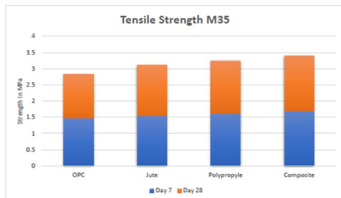
Fig -3.5 Tensile Strength M35
