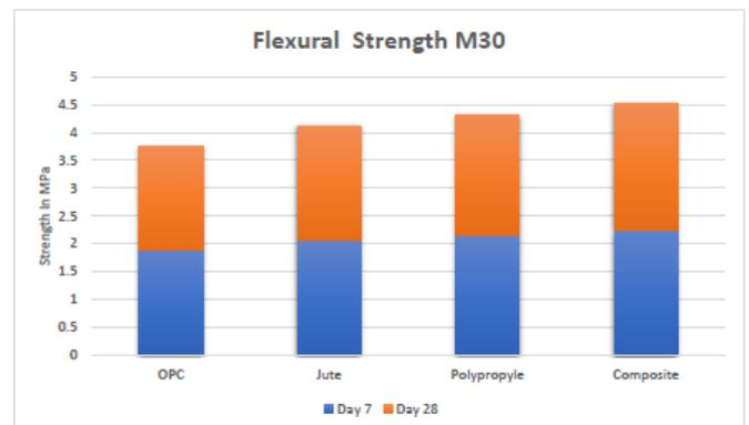
Fig -3.1 Value of Flexural Strength M30
