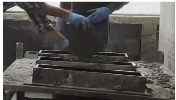
Fig -2.4: Filling molds in 3 layers
