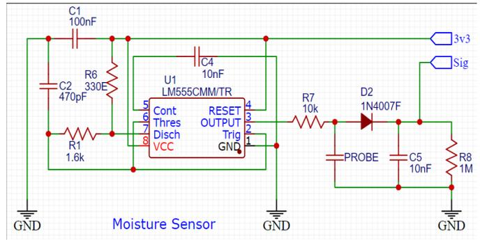
Fig -6: Capacitive moisture sensor circuit diagram
