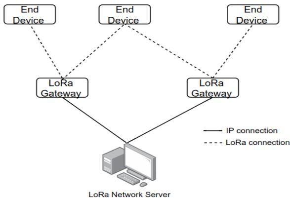
Fig-2: LoRaWAN Architecture
