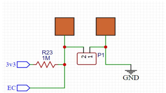
Fig-7: Electrical Conductivity sensor circuit.
