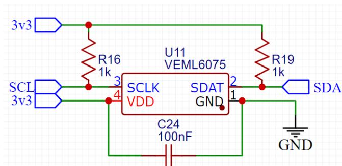
Fig-8: UV detector circuit diagram
