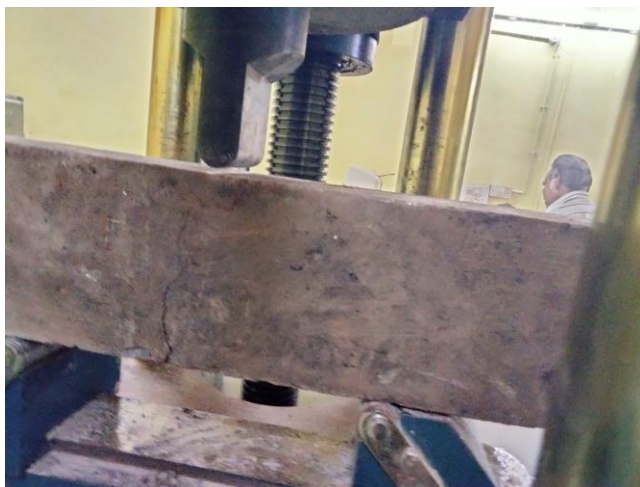
Fig-4: flexural strength test in universal testing machine.
