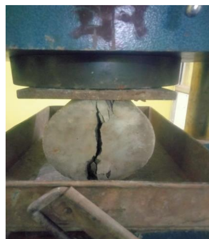
Fig- 3: Split tensile strength test in Universal testing machine.
