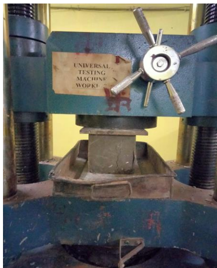
Fig-2: Compressive strength test in Universal testing machine.
