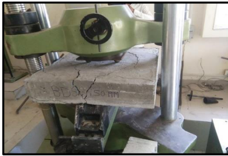
Fig.13. Slab Failure at maximum Load.
