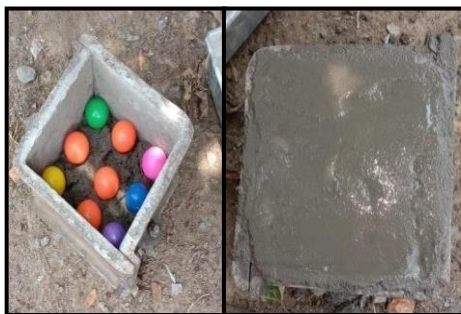
Fig.4 Placing of Bubbles and Casting
