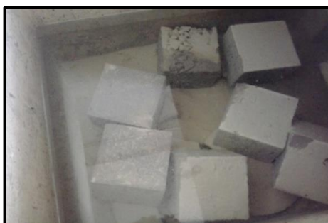
Fig.5 Curing of Cubes
