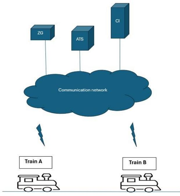
Fig -1: Basic Structure of Communication in CBTC
