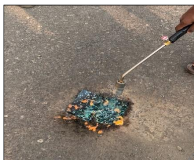
Fig- 10: Melting the HDPE Plate
