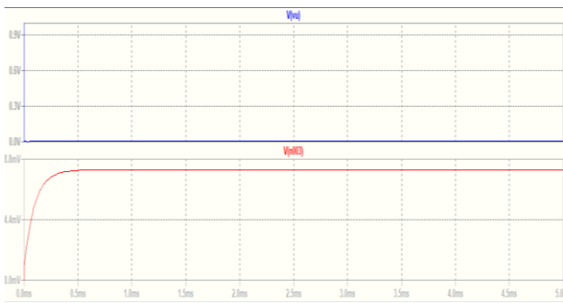
Fig14 output voltage of the follower circuit when the input voltage of -19V
