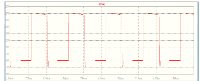
Fig9 voltage waveform across the switch during CCM
