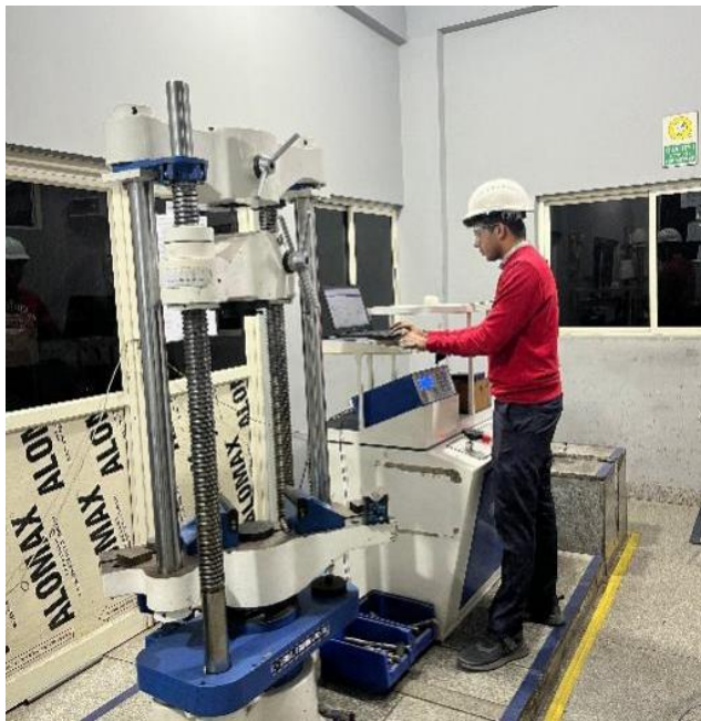
Fig -5: Machined test bars are tested in universal Testing Machine (UTM)
