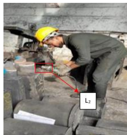
Fig -2: Samples taken from edge of casting, below the riser L 2
