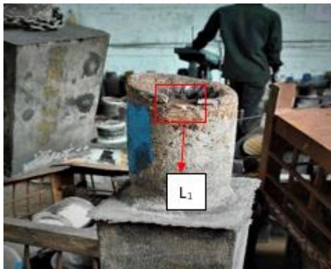
Fig -3: Samples taken from edge of casting, riser region- L 1
