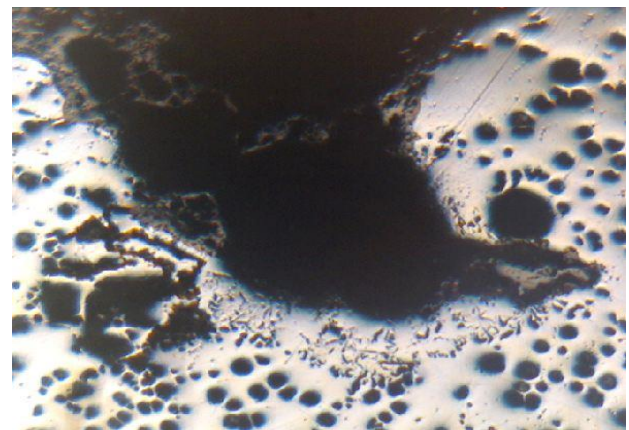
Fig -8: Unetched Micro-image of a sample from riser area L 1 at 100x
