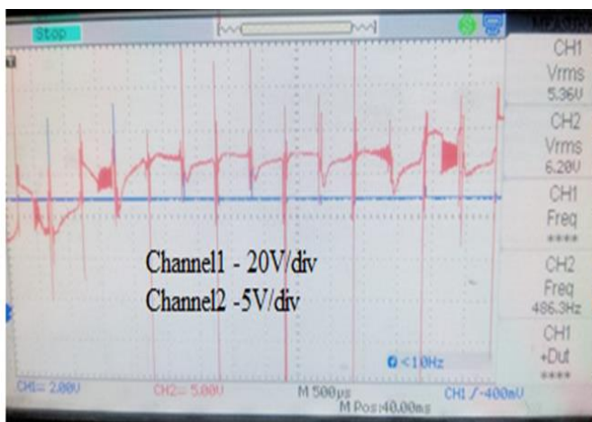
Fig-14 The load voltage along with battery voltage when battery is charging
