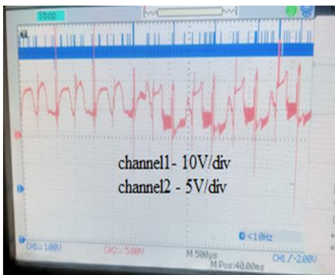
Fig-15 The load voltage along with battery voltage when battery is discharging
