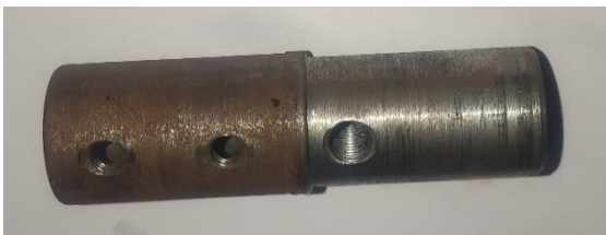
Fig.11. Steering column and pinion couple
