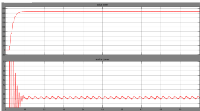
Figure 6: Inverter Power Waveforms
