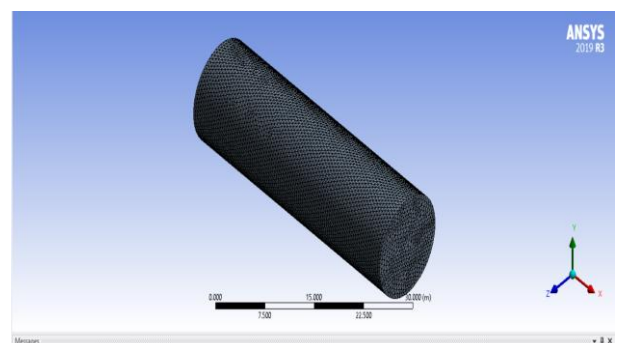
Figure 9. 3D mesh model of outer tube
