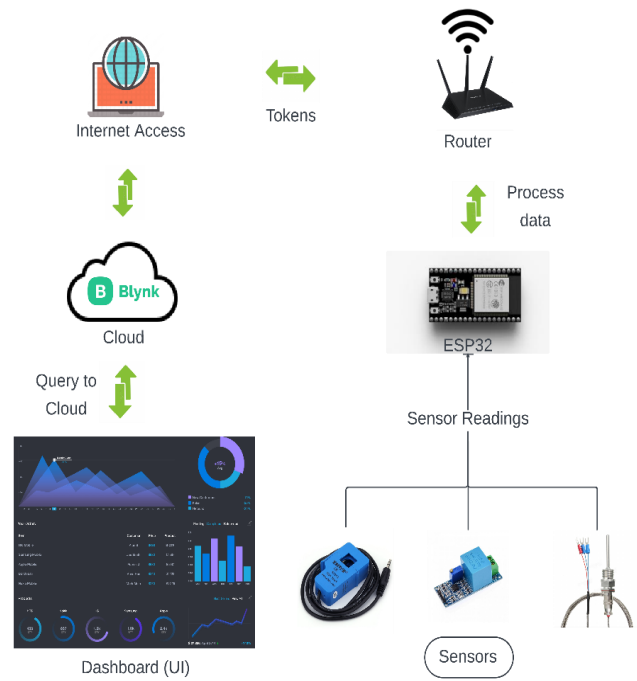
Fig -3: System Architecture
