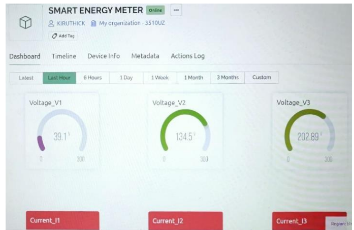
Fig -6: Blynk dashboard displaying real-time data.
