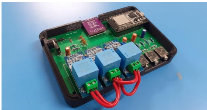
Fig -5: Final Prototype enclosed in a 3D-printed case
