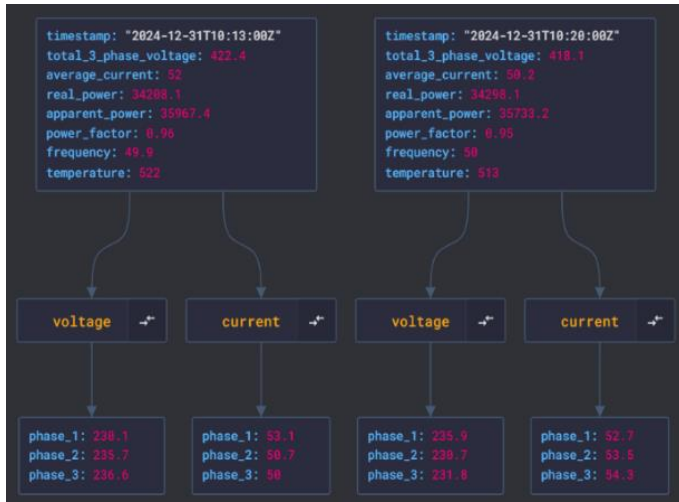
Fig -7: JSON log data for performance analysis
