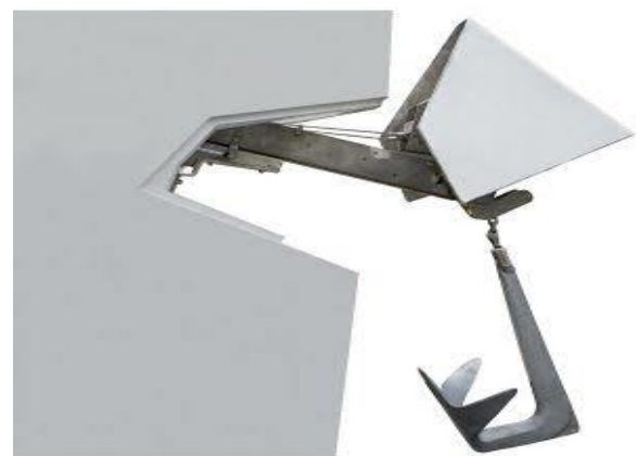
Fig: 2 Anchor with enclosing door
