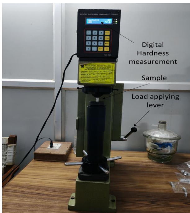
Fig -1: Rockwell Hardness Setup
