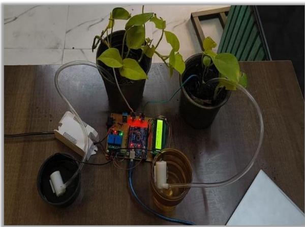
Fig 2. Experimental setup of the automated irrigation system.
