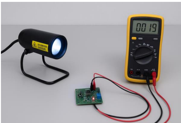
Figure 3. Experimental setup for circuit testing This figure shows the setup used for testing the UV detection circuitry. The calibrated UV lamp provided a source of controlled radiation, while the digital multimeter measured output voltages that corresponded to different intensities of UV radiation. The setup validated the comparator's response accuracy and sensor sensitivity under various conditions of light exposure.
