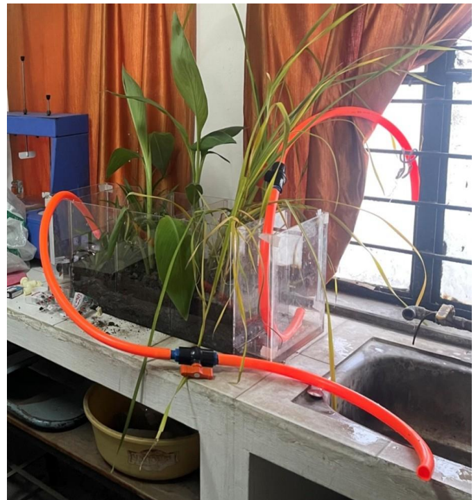
Figure 7.3: Photograph of working RZT model
