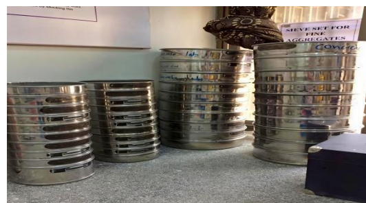
Figure 1: Standard sieve set used for fine aggregate gradation.
