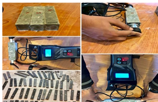
Figure 7: Ultrasonic pulse velocity (UPV) test setup.
