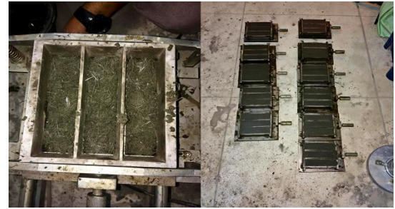
Figure 4: Prismatic steel molds (40×40×160 mm) and fresh fiber-reinforced mortar.
