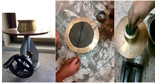
Figure 6: Flow table used for workability measurements.
