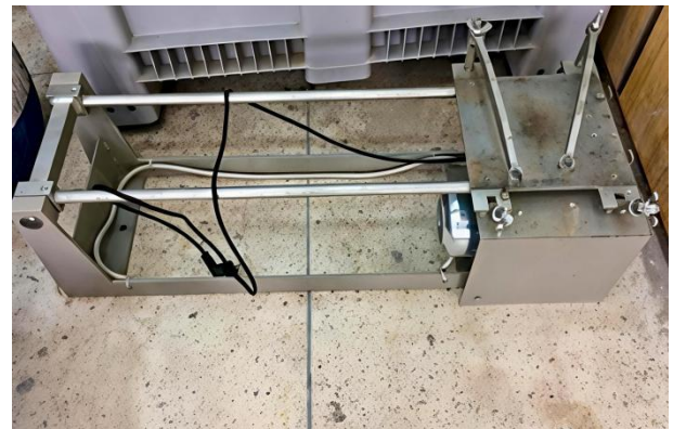
Figure 5: Mechanical jolting machine used for specimen compaction.
