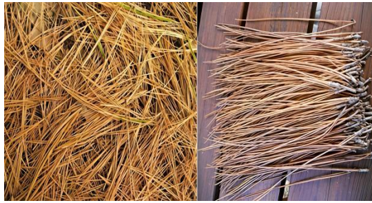
Figure 3: Pine needle fibers: raw needles (left) and processed fibers (right).
