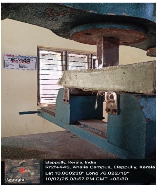
Fig -2: Flexural strength test of GFRP bonded concrete beam.
