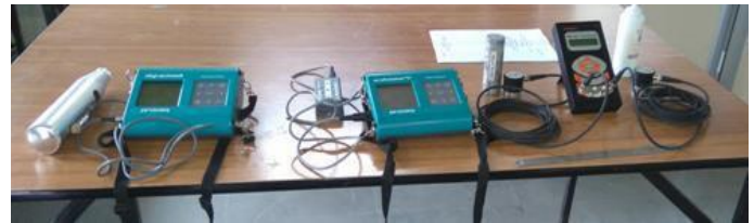
Fig.(4) Ultrasonic Pulse Velocity Test Setup
