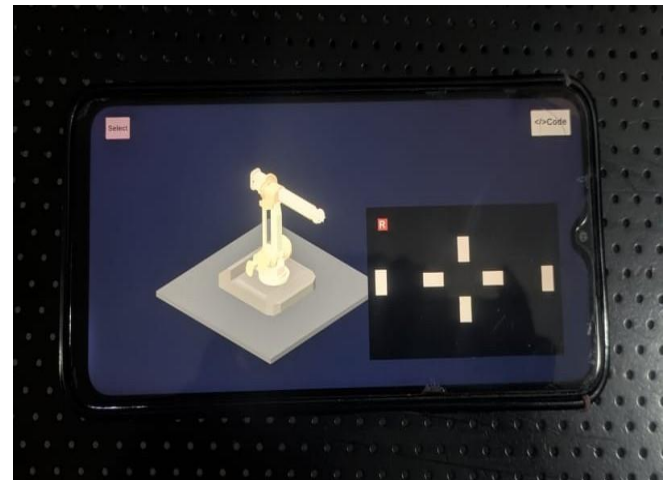
Fig -6: Mobile Based Controller with Feedback system in 3D Model
