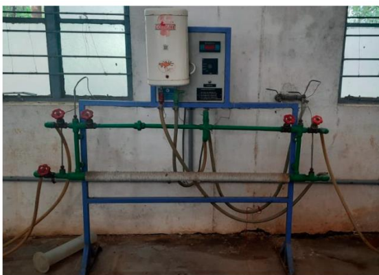
Figure 3.11 Experimental setup of double pipe heat exchanger
