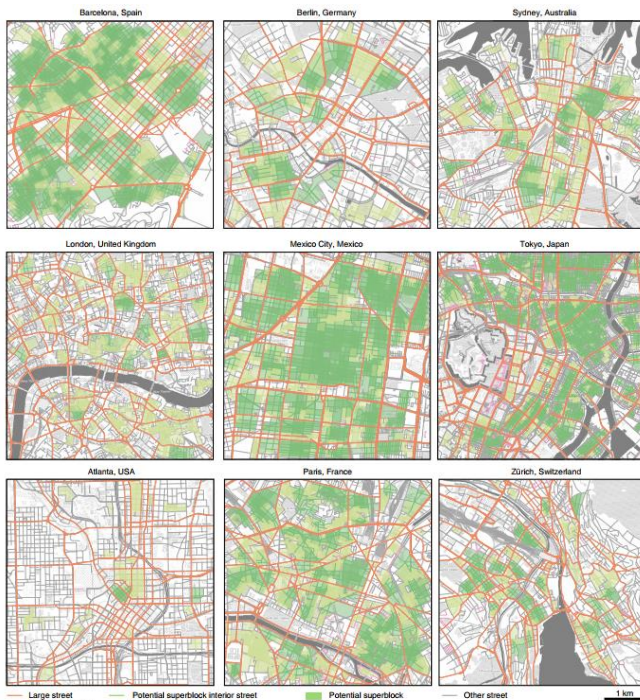
Fig -3: Modelled classification of the street network for selected cities. source: Nature sustainability research paper
