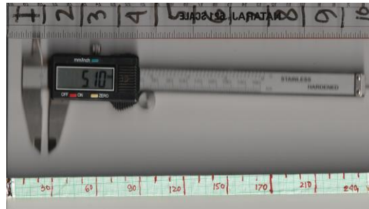
Fig- 3 ; Measuring instruments, Digital Vernier Caliper, Scale and specially designed simple millimeter scales, for measuring color-chromato level size
