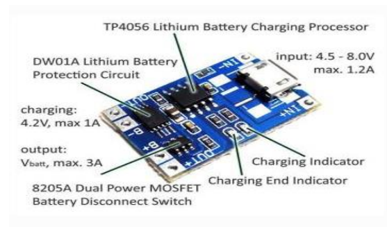
Fig.4: TP4056 charging module
