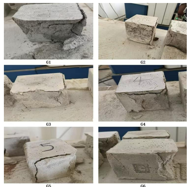
Fig-4 : Failure Modes of Specimens with Varying RHA-SF Substitution Ratios
