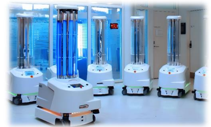
Fig -1: Ultraviolet sterilization by robots in different departments in hospital [8].
