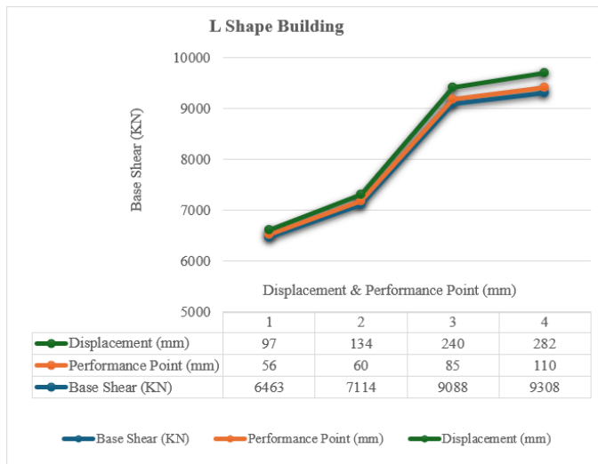
Chart 3: Chart shows the relation of base shear vs displacement & performance point for L Shape Building.
