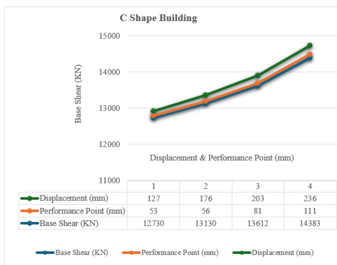
Chart 3: Chart shows the relation of base shear vs displacement & performance point for C Shape Building.
