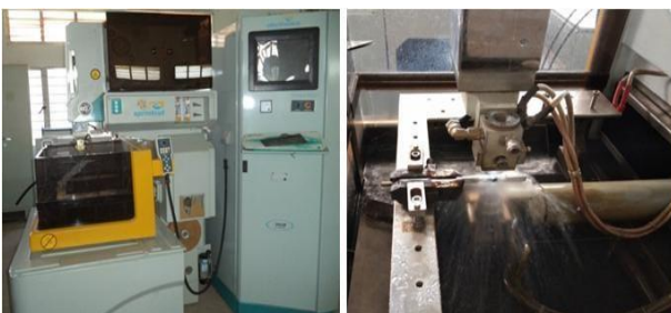
Fig 4.2 Computer numerical controlled wire electric discharge machining and the machining chamber.
