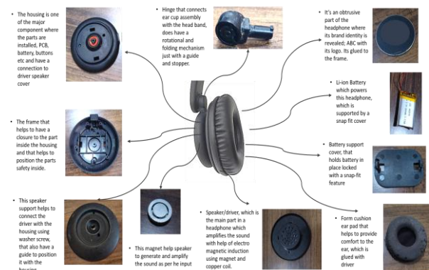
Fig -8: LH Ear Cup assembly of ABC Headphone
