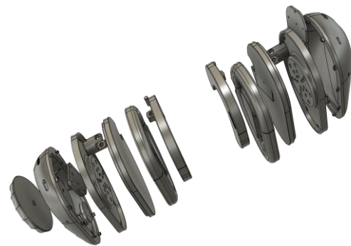
Fig -26: Exploded view of redesigned headphone
