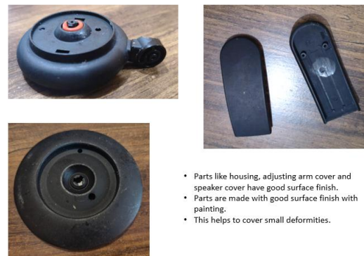
Fig -19: Surface finish of headphone parts
