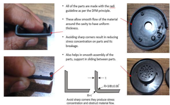
Fig -23: Radii and Fillets ensured on headphone parts
