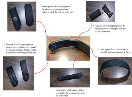
Fig -7: Headband assembly of ABC Headphone
