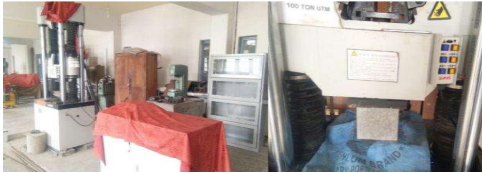
Figure 1: Universal Testing Machine for Compressive Strength Test
