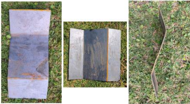
Fig. 2: Model sheet pile used for reinforcement
