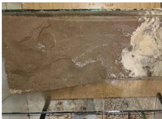
Fig -4: Measuring displacement of soil without sheet pile
