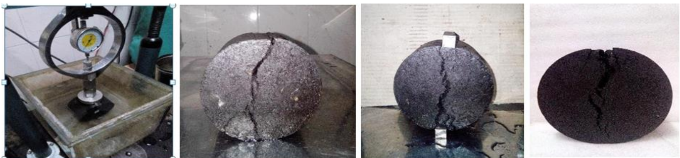
Figure 3.8 Loading and Failure Pattern of Indirect Tensile Strength Test
