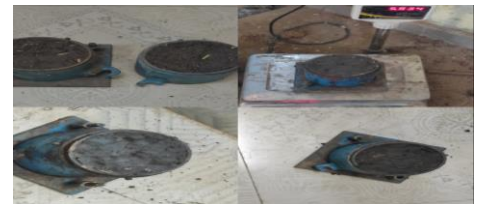
Figure 1: (c) Soil- Fibre Proctor test
