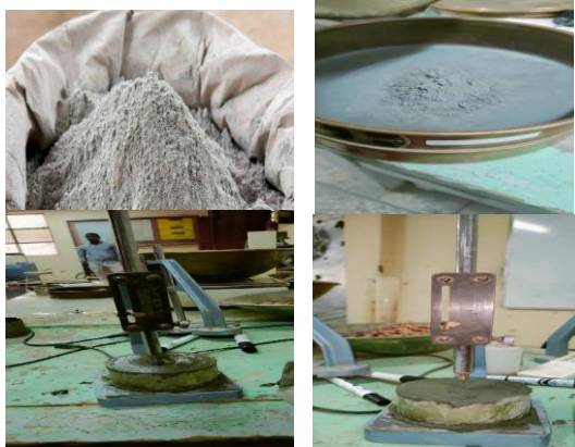
Fig -1: cement and tests equipment's
