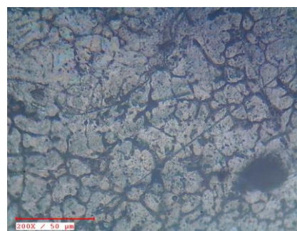
Fig. 12: Microstructure of Al7178 + 2% SiC + 2% B 4 C at 200x Magnification
