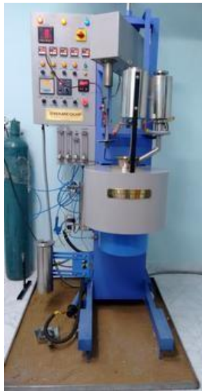
Fig. 5: Stir Casting Setup
