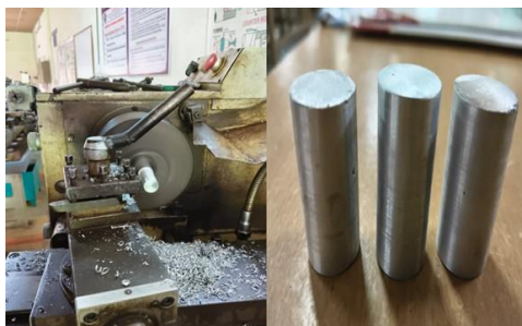
Fig. 8: Machining of Composite Specimens
