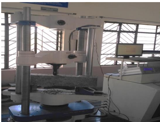
Fig 3.4.1 : Flexural strength testing
