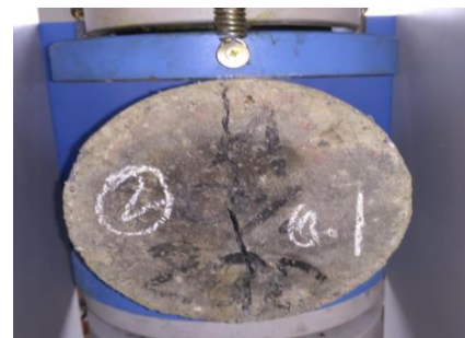
Fig 3.3.1 : Split tensile strength testing
