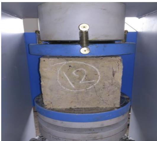
Fig 3.2.1 : Compressive strength testing
