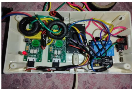
Fig. 1. Internal assembly showcasing the integration of the ESP32 microcontroller, PZEM sensor module, and the relay control board.
